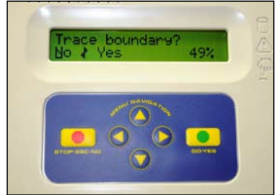
Figure 9. NEW FEATURE (Trace Boundary)
