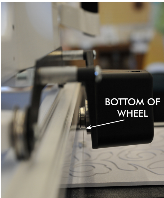
FIGURE 11. Drive wire wrapped on drive wheel
