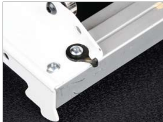
... Y-axis wire holder installed, note orientation
