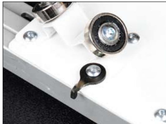
... Y-axis wire holder installed, note orientation
