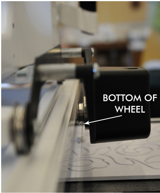
FIGURE 9. Y-Axis Drive Wire Installation
