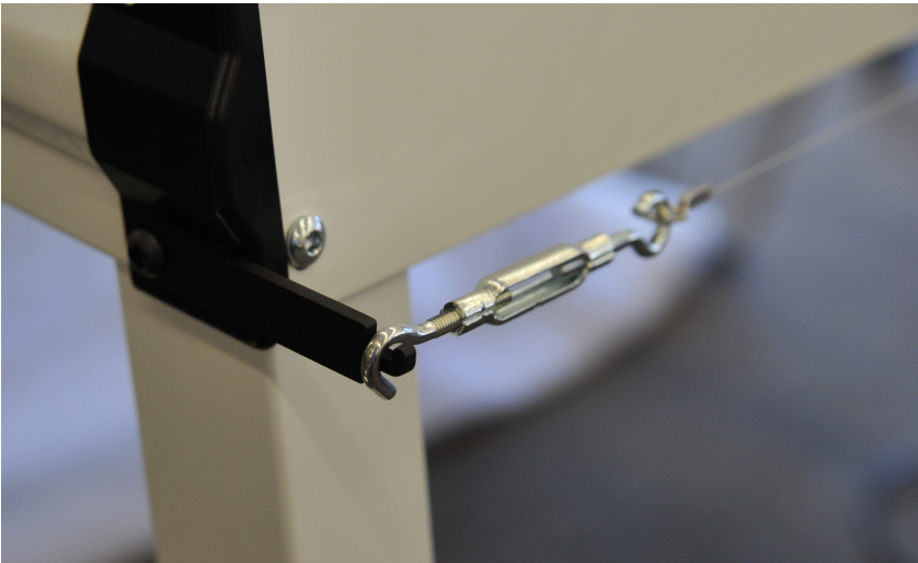
FIGURE 7. X-Axis Turnbuckle Installation
