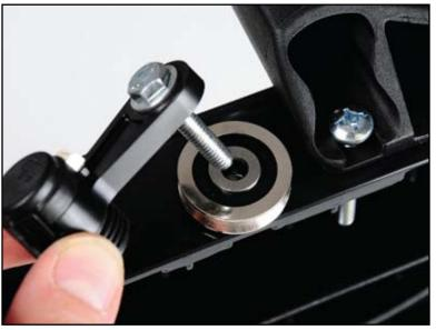
If you have the Quilter's Cruise Control<sup>®</sup> installed, remove the optical encoders from the upper and lower carriages at this time. Re-install the bolts to secure the wheels to the carriages
