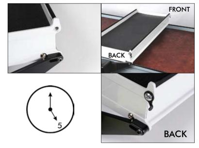
Remove the second screw that is at the top of the opposite end of the lower carriage on the same side. Attach the second Y-axis wire holder and replace the screw. Tighten securely ensuring that the hook on this wire holder is in the 7 o'clock position.
