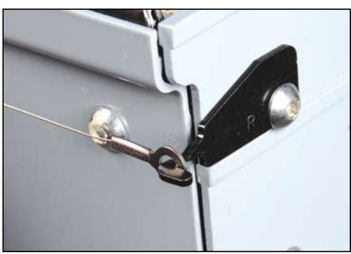
Take one end of the lower drive wire and place the eyelet around the hook of the right X-axis wire holder.
