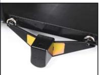
Next, place the second  $1\frac{1}{2}$ " button head screw into the slot in the assembly. Slide on a washer from the QBOT installation hardware pack, metal wheel, and  $3^{rd}$ washer. Insert into the upper carriage and screw gently into the original nut. Securely tighten both screws after the assembly is in place on the carriage.
