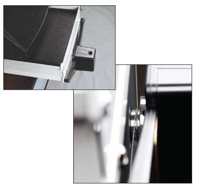
Lift the whole carriage unit off the rails and move slightly to the back of the frame. Standing at the back of the frame, place the lower drive wire over the drive pulley, **wrapping down and around twice**. Holding the wire taut with your left hand, return the carriage back to the rails of the frame. The photo to the left is a view looking down on the drive assembly.
