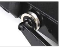
Place one  $1\frac{1}{2}$ " button head screw through the hole of the drive assembly, replace one metal wheel, then slide on a washer from the QBOT installation hardware pack. Insert into the rear hole in the upper carriage and screw gently into the original nut that is in the upper carriage. Do not tighten at this point.
