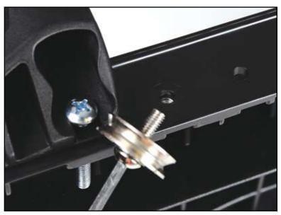
Attach the second drive assembly to the right hand side of the upper carriage as viewed when you are standing at the back of the frame. Set the upper carriage on its side with the handle holder of the carriage on the left. Remove both bolts and metal wheels from the right side. Set aside the wheels to be used later. The bolts and washers that were removed will not be reused.
