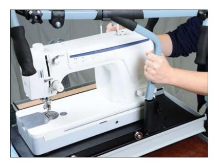
Remove the handle assembly and set aside. Unplug all cords from the sewing machine, then lift it off of the upper carriage. Carefully place the machine in a convenient location.
