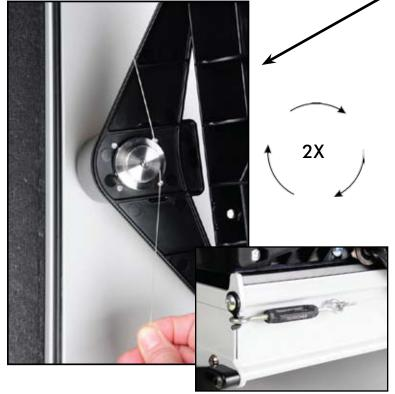
Take one end of the 24" wire and place the eyelet around the hook of the Y-axis wire holder on the front of the lower carriage.
