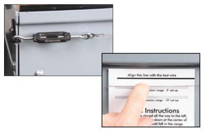
Attach the tensioner to the hook of the left X-axis wire holder. Attach the eyelet of the wire to other end of the tensioner. Tighten the wire with the center of the tensioner until it is stretched like a guitar string. Use the tensioning template as your guide for tightness as before.
