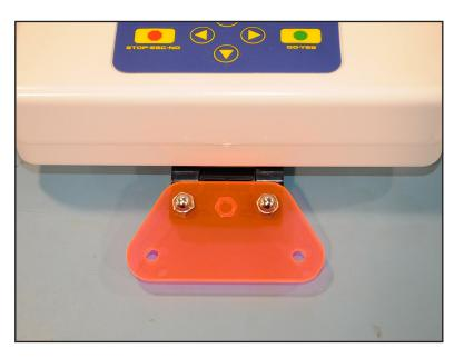
Finally, remove the attachment bracket that came with your QBOT and replace it with the one from this kit as shown to the left.
