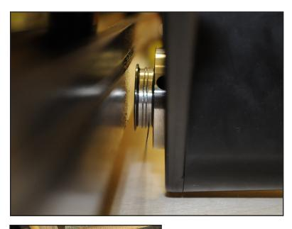
Finalize the installation of the Y-Axis drive assembly by installing the drive wire. THE DRIVE WIRE MUST BE WRAPPED SO THAT THE WIRE ENTERS AND EXITS FROM THE BOTTOM OF THE DRIVE WHEEL AS SHOWN IN THE PICTURE TO THE LEFT.
