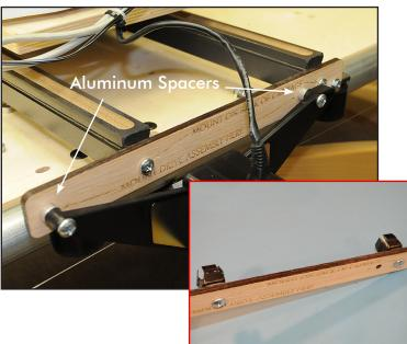
Next, remove the plastic caps from the back end of the lower carriage tubes. Tap the tube nuts provided into the ends of the tubes. The X-Axis drive bracket will attach to these nuts with (2) 11/2" long screws. The pictures to the left show the drive bracket attached to the tube nuts and when the assembly is installed on the carriage.
