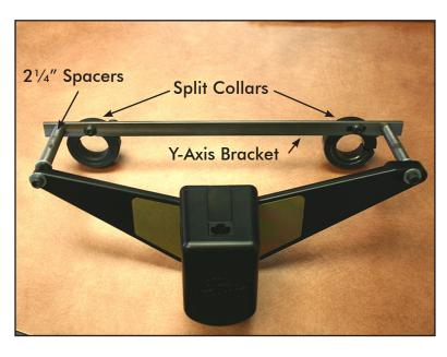
Next, secure the Y-Axis drive assembly to the Y-axis bracket provided using (2)  $3\frac{1}{2}$ " screws, (2)  $2\frac{1}{4}$ " spacers, (2) washers, and (2)  $\frac{1}{4}$ " nuts.
