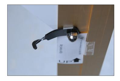
The final step of the drive system assembly is installing the X-Axis drive wire. If your frame is set up at the 5 foot length, use the blue-wrapped wire from your QBOT wire pack. If your frame is set up at the 10 foot length, use the redwrapped wire.
