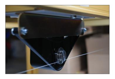
Connect the eyelet at the other end of the drive wire to one end of the tensioner. Connect the other end of the tensioner to the X-Axis bracket at the opposite side of the quilting frame. Use the tensioning template from the back of the QBOT manual as a guide to adjust the tension in the wire.
