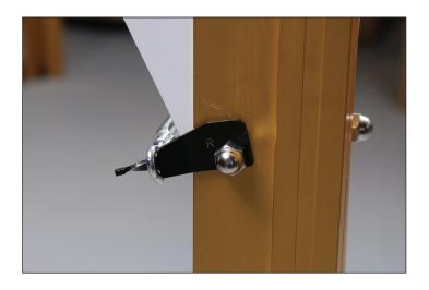
Slide the eyelet of one end of the drive wire over the X-Axis wire holder and while keeping the wire taut, wrap over the X-Axis drive wheel the following number of times:
