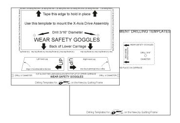
The first step to installing the QBOT on the NewJoy quilting frame is to drill holes in the upper and lower carriages. First, cut out the templates on pages 7 and 8 of these instructions.
