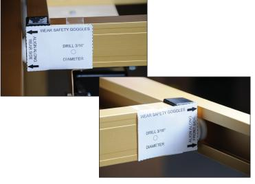
Using the drilling templates for the Y-Axis wire holders from page 8 of these instructions as a guide, drill two 3/16" diameter holes in the lower carriage as shown in the photos to the left.
