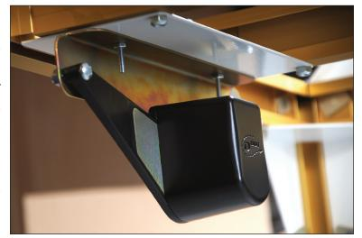
Next, install the X-Axis wire holders to the rear outer frame legs as shown in the pictures to the right. Temporarily remove the acorn-style nut and place the X-Axis wire holders using the alignment templates from page 7 of these instructions. The orientation of the X-Axis wire holders should match the angle of the templates. Secure with the acorn-style nuts.
