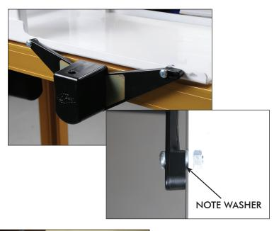
Mount the drive assembly to the upper carriage using two 1/4" screws and nuts. Use one 1/4" washer from your QBOT hardware kit on the slotted end of the drive assembly as shown in the photo to the left.
