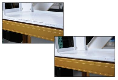
Next, use the other drilling template from page 7 of these instructions to drill two 1/4" holes in the upper carriage of your frame. Align the template as shown in the photo to the left and drill the holes. Remember to wear safety goggles when drilling the holes.
